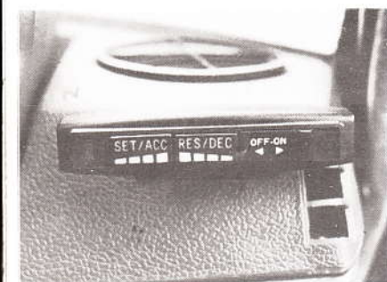
Left: After-market cruise control wasn't connected
